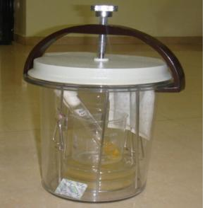
Fig. 6: Anaerobic Chamber
