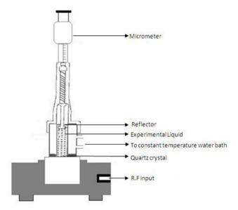
In an ultrasonic interferometer, the ultrasonic waves are produced by the piezoelectric method. In a fixed frequency variable path interferometer, the wavelength of the sound in an experimental liquid medium is measured, and from this one can calculate its velocity through that medium.
