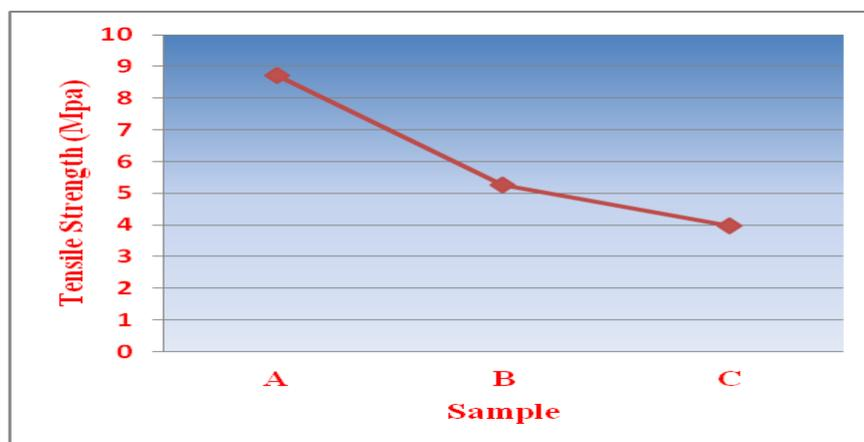
**Figure 1: Variation in mechanical strength with varying ratio of starch and PVA in the blend**
