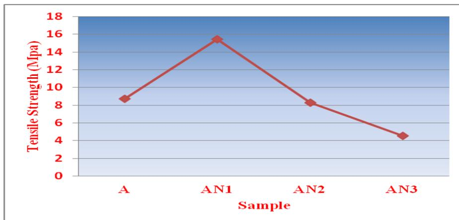
**Figure 3: Variation in Mechanical strength with increasing filler loading**
