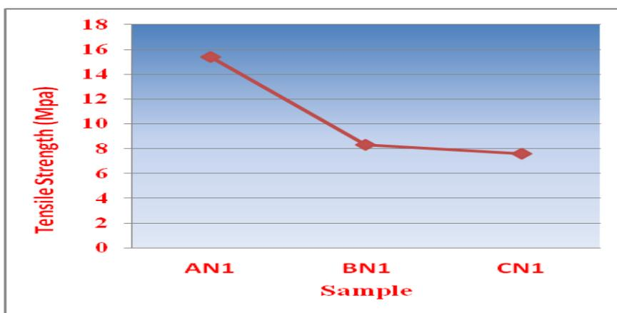
**Figure 2: The Change in Mechanical strength in 1% clay filled sample of starch and PVA blend with varying blend ratio**
