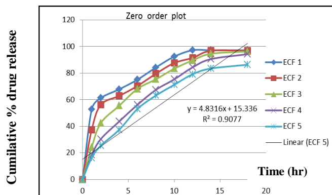
Figure No.4 : Zero Order Plots of Quetiapine Fumarate Pellets prepared by Fluidized bed Coating Process
